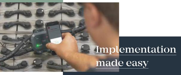
Using the NFC interface, the TagID can be configured quickly and easily via the TagID Config app. The user-friendly interface of our app assists in entering the few necessary parameters. The TagID automatically checks whether the voltage value entered during configuration matches the actual measured value. Deviations are detected immediately and consequential damage is thus effectively prevented.
