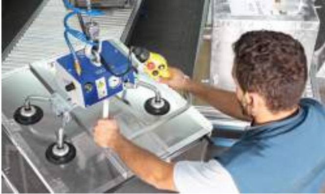
VacuMaster Light for handling metal housings
