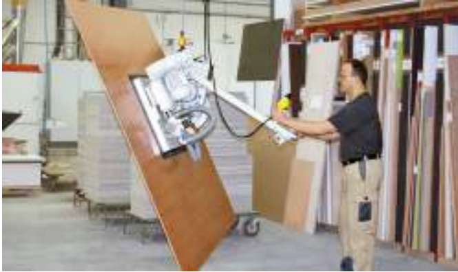
VacuMaster Multi for swiveling wooden boards by 90°
