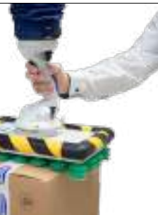
Multiple vacuum gripper Universal gripping of various cardboard box sizes and qualities with a minimum occupancy rate of 75 %.
