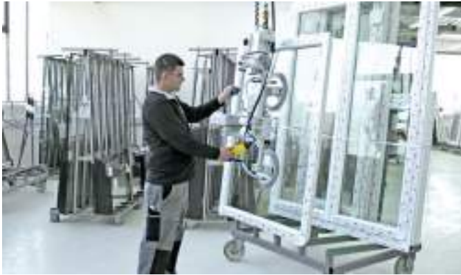
VacuMaster Window for rotating and palletizing windows
