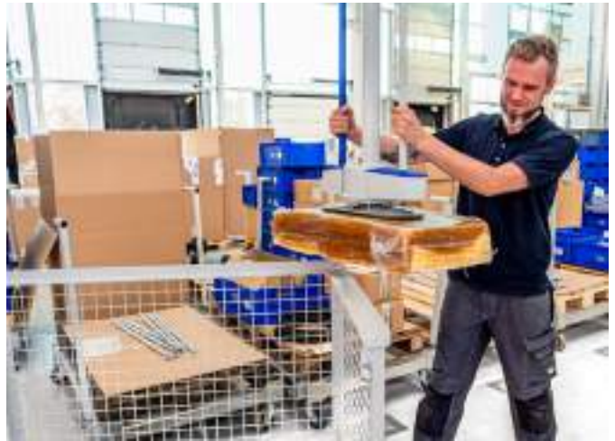
Vacuum tube lifter Jumbo Low-Stack for handling raw rubber bales
