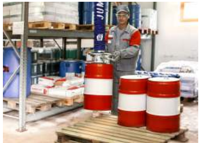
Vacuum tube lifter JumboSprint for handling barrels
