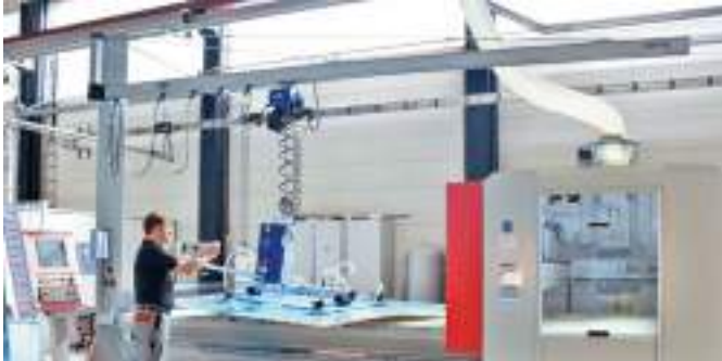
Column-mounted jib crane SK with chain hoist and lifting device VacuMaster
