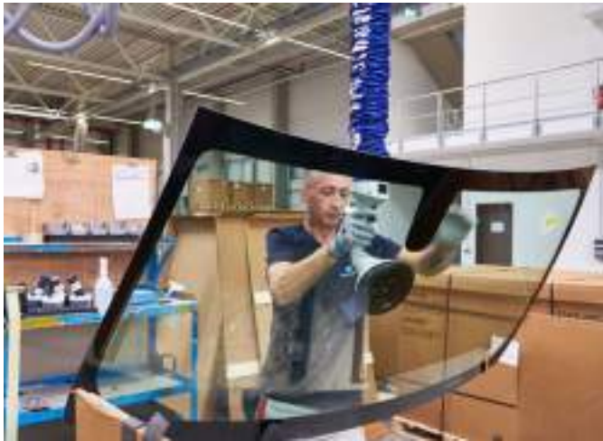
Vacuum tube lifter JumboFlex for handling windshields
