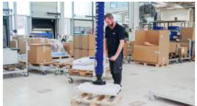
JumboFlex High-Stack when handling bags
