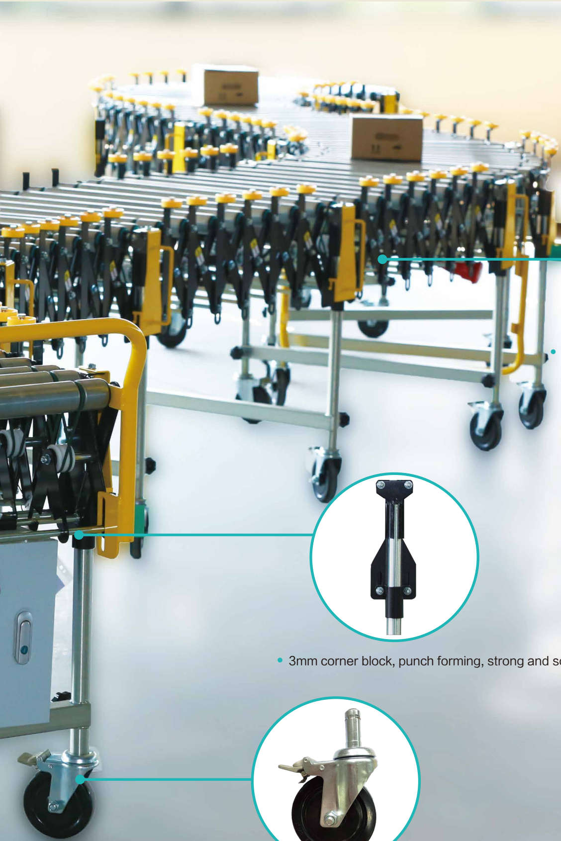
• OD125mm nylon brake castor, firm and reliable.
