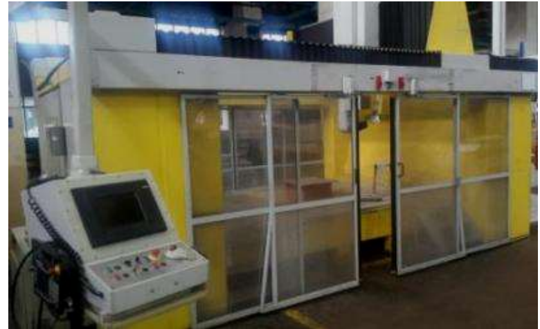
Bayardon - 5 Axis CNC Trimming machine :
