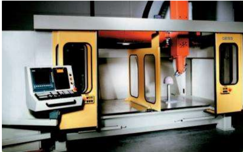
Geiss - 5 Axis CNC Trimming machine :
